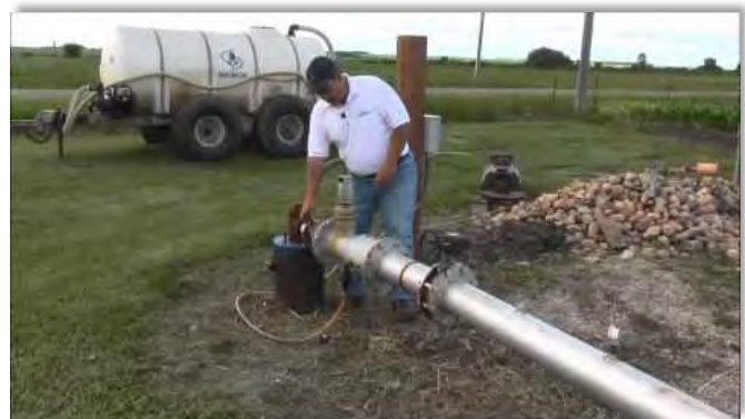
View of fertigation system with check valves and portable tank.
